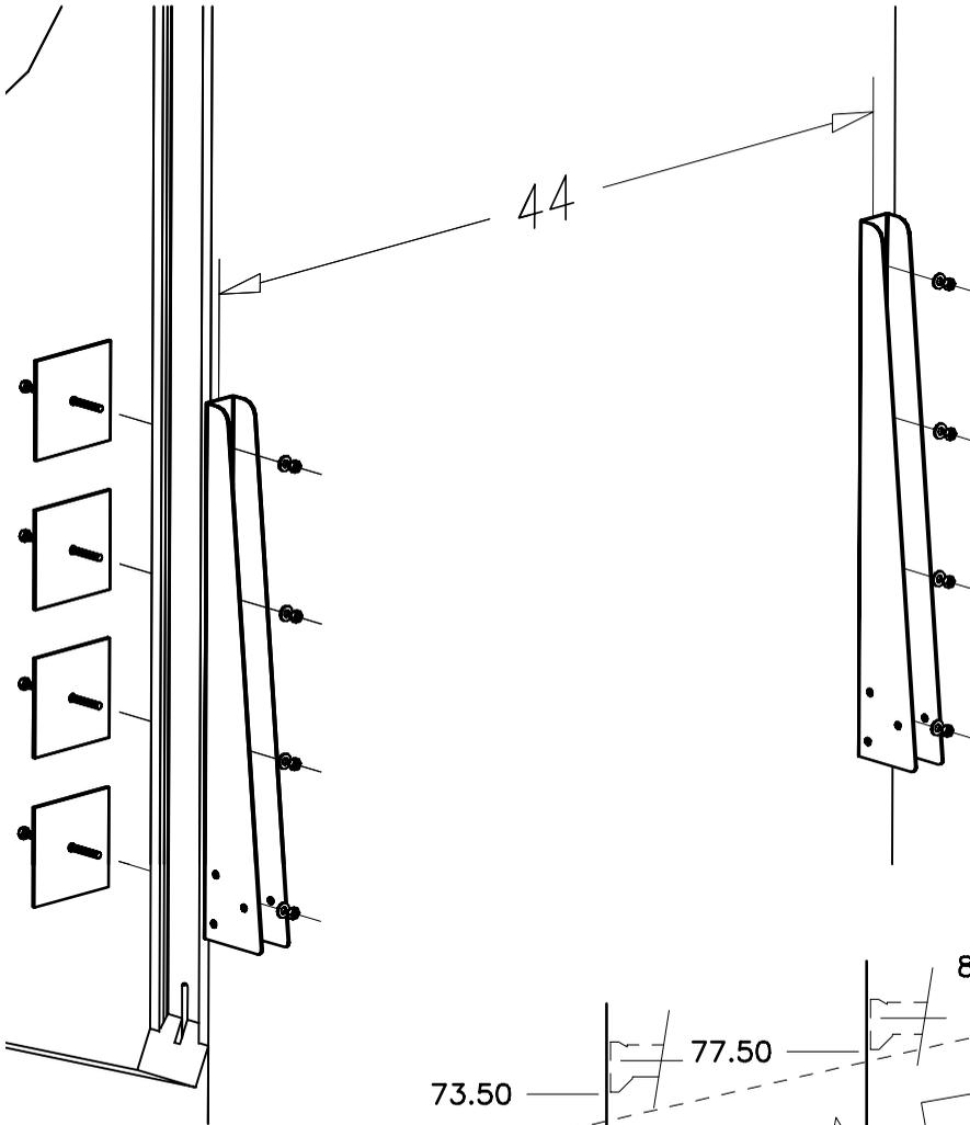
FIND THE LOCATIONS OF YOUR PANELS' STRAPS AND POCKETS ON THIS DIAGRAM. DO NOT DRILL CLOSE TO THESE ELEVATIONS.
